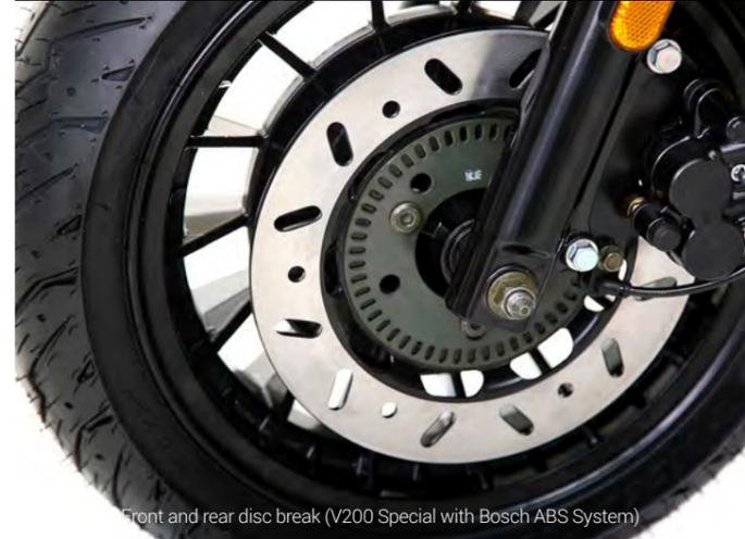
Front and rear disc brake (V200 Special with Bosch ABS System)
